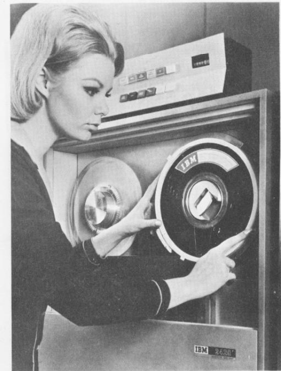
Figure 79. Tape Reel cartridge operation
